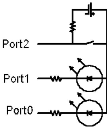
And here is how to wire up the LEDs on the breadboard (you will have to figure out how to wire the switch).
