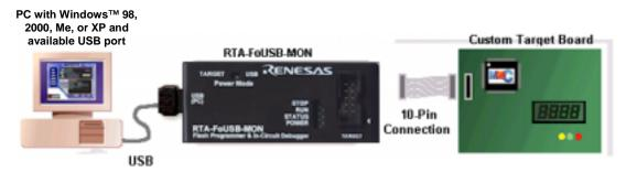
Figure 1 ICD System Connectivity
