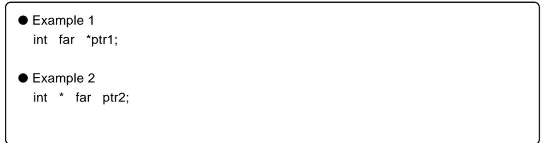
Figure B.7 Example of Declaring a Pointer Type Variable(1/2)
