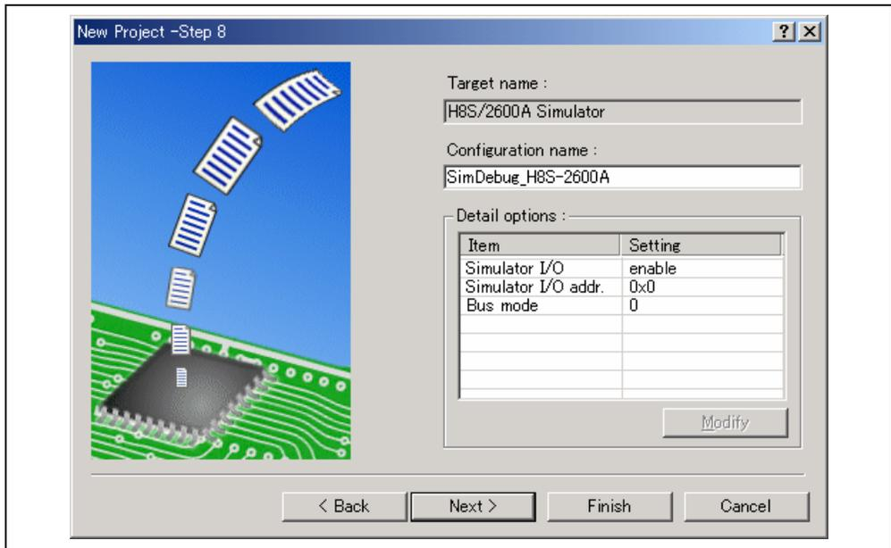
**Figure 3.9 Debugger Option Setting Display (Step 8)**
