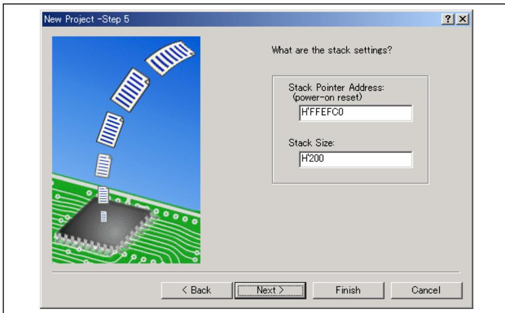
**Figure 3.6 Stack Area Setting Display (Step 5)**
