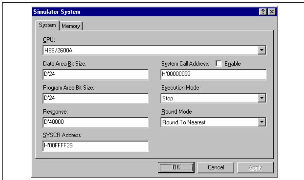
**Figure 4.86 Simulator System Dialog Box (System Tab)**
