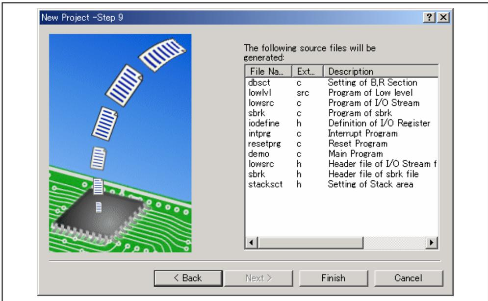
**Figure 3.10 Generation File Name Modification Display (Step 9)**
