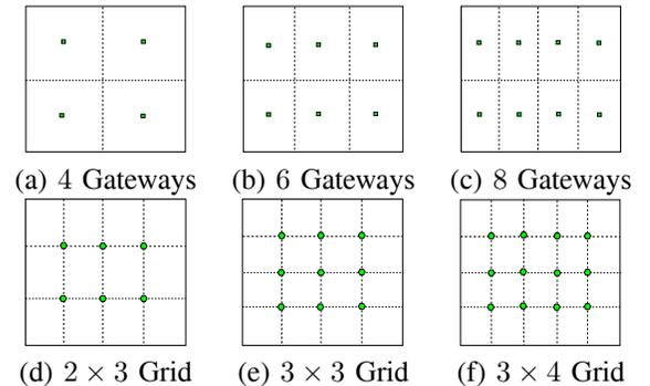
Fig. 4. The layouts of gateways in fixed deployment scheme (a-c) and the grids used in our deployment scheme (d-f).
