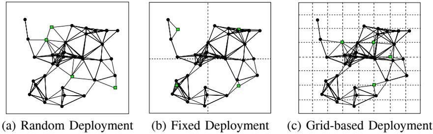
Fig. 3. Three gateway deployment methods: 4 gateways (grey square) are deployed in a mesh network with 33 mesh nodes (black dot).
