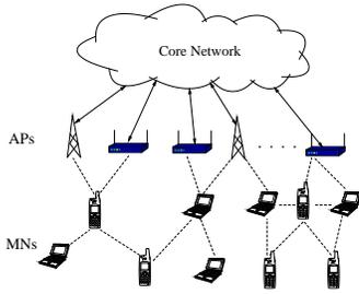
Fig. 1. Network Architecture of Heterogeneous Access Network.
