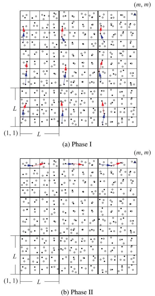
**Fig. 3** Our collection method: Phase I: each node sends its data to its upper cell; Phase II: each node in the top row sends its data to its right cell.
