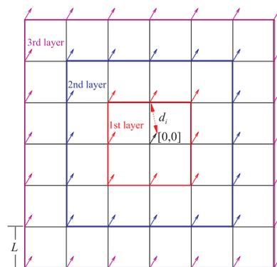
**Fig. 2** Grid partition of interference blocks with size of  $L \times L$  and simultaneous transmissions around the center block  $[0,0]$  by layers.
