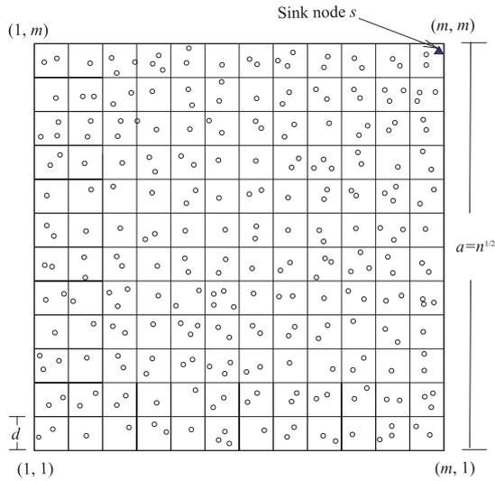
**Fig. 1** Grid partition of the sensor network:  $m^2$  cells with cell size of  $d \times d$ .
