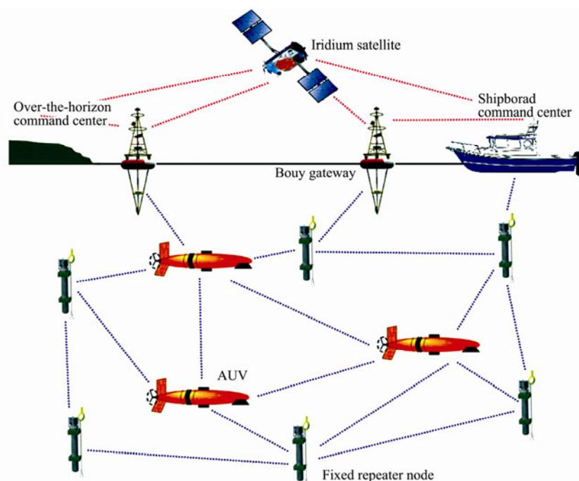
Fig.1 Seaweb network in the Eastern Gulf of Mexico, including three AUVs, six repeater nodes, and two gateway buoys (Rice, 2007).
