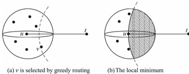
Fig.6 Illustration of 3D greedy routing.
