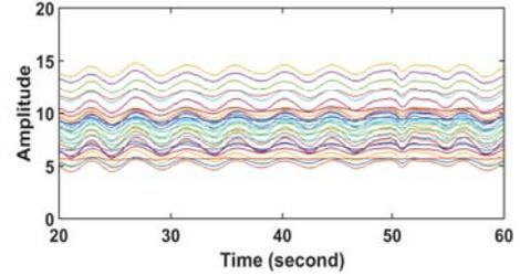
(b) 2D CSI time series after passing low pass filtering
