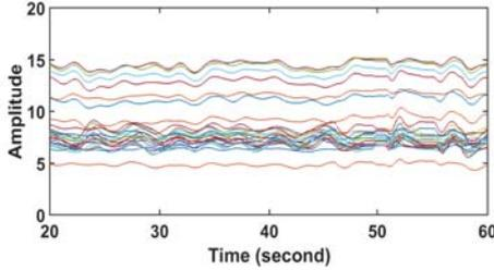
Figure 6. CSI time series influenced by a moving target.
