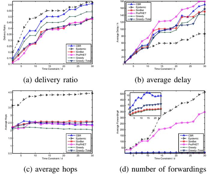
Fig. 6. Simulation results of all different routing algorithms (over MIT data set) with 3 copies of message.
