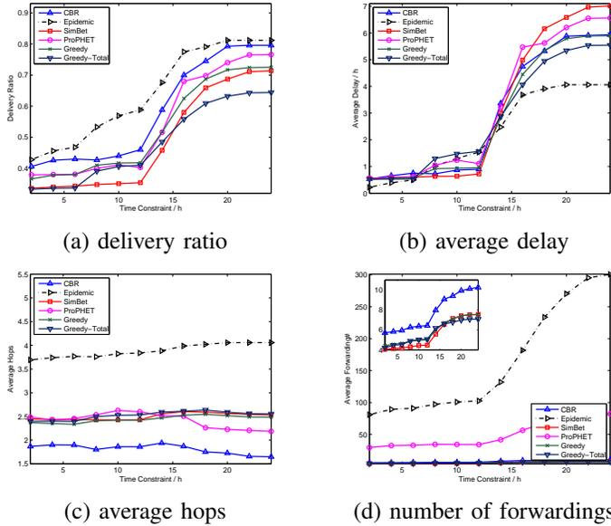
Fig. 5. Simulation results of all different routing algorithms (over InfoCom 2006 data set) with 3 copies of message.
