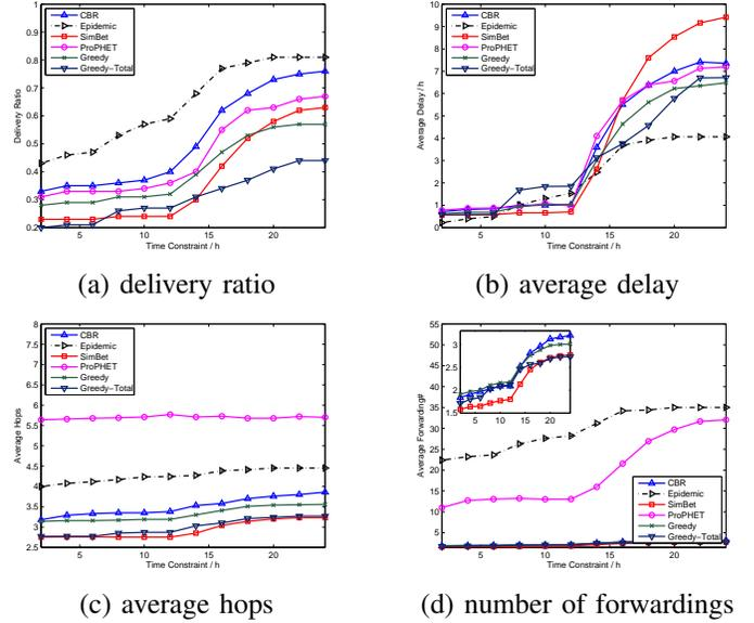
Fig. 3. Simulation results of all different routing algorithms (over InfoCom 2006 data set) with single copy of message.
