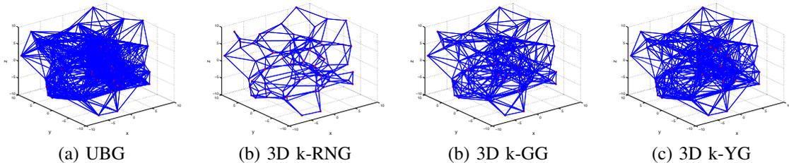
Fig. 3. 3D localized topologies which are constructed from the same UBG. Here,  $n = 100$ ,  $k = 2$  and  $P^{max} = R^2 = 81$ .
