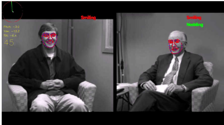
Fig. 1. An example of the automated analysis for human Nonverbal Communication Computing [2]. Sample snapshots from tracked facial data showing an interviewee (left) and an interviewer (right). Red dots represent tracked facial landmarks (eyes, eyebrows, etc.), while ellipse in top left corner depicts the estimated 3D head pose of the subject; top right corners show the detected expressions and head gestures for subject and interviewer.
