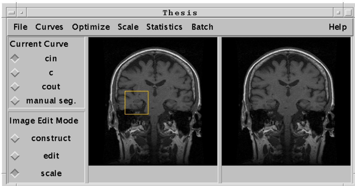
Figure 4.3 Image scale bounding box. The box in the image above identifies the region that the scaling operation will act upon.
