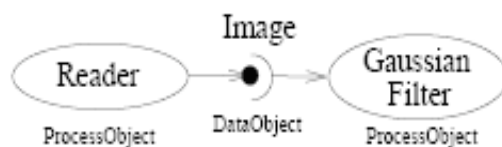
Figure A.3. Relationship between ProcessObject and DataObject
