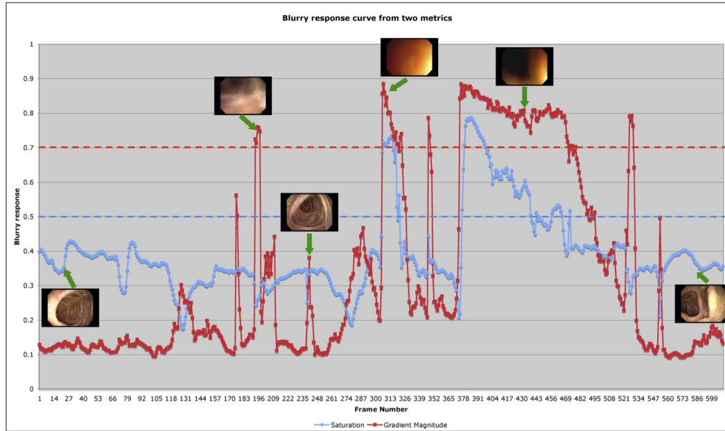
Figure 5.4: Results of blurry image detection based on edge and saturation filters. Solid red and blue lines represent the response curves of edge and saturation filters, respectively. Thresholds 0.5(saturation) and 0.7(edge) are used for these two filters, corresponding to blue and dash lines.
