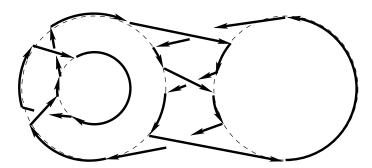
The Seifert circles of an oriented link diagram are obtained by smoothing all crossings.
