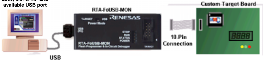
Figure 1 ICD System Connectivity
