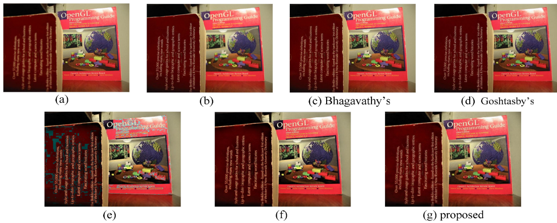
Fig. 5. Multi-focus color image fusion: book. (a)(b) are sources, (c)(d)(g) are fusion results by Bhagavathy's [12], Goshtasby's [3] and the proposed method, (e)(f) are fusion results with color distortion.
