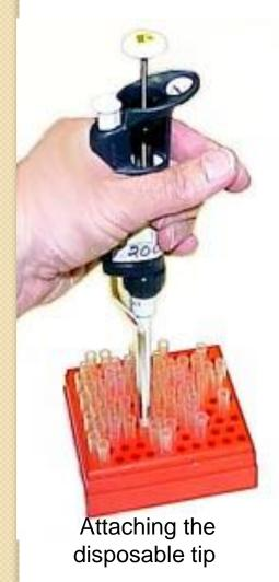
Tip boxes are labeled for the range of barrel they accommodate (there are some manufacturer-specific types so check if you are mixing and matching).
