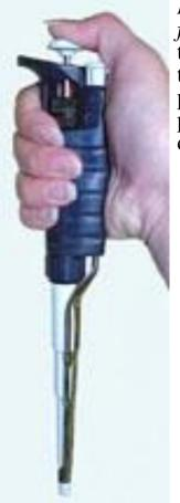
Depress the plunger first: don't put the tip in the liquid and then depress the plunger (the pressure is different).
