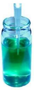
The tip must be below the surface of the liquid throughout the process of pulling up the liquid.
