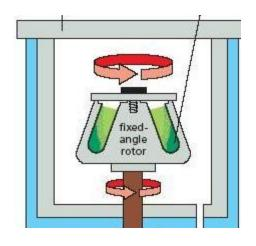
If the tubes across from each other not balanced (by mass) the rotor will start to rock, and can eventually break.
