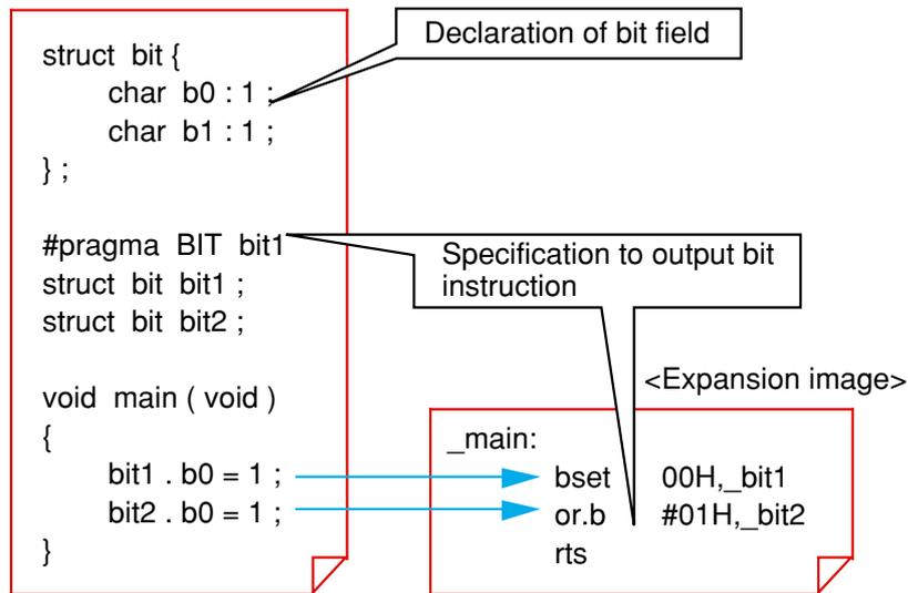
**Figure 2.3.7 Typical description of "#pragma BIT"**
