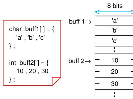
Figure 1.7.2 Declaration of one-dimensional array and memory mapping
