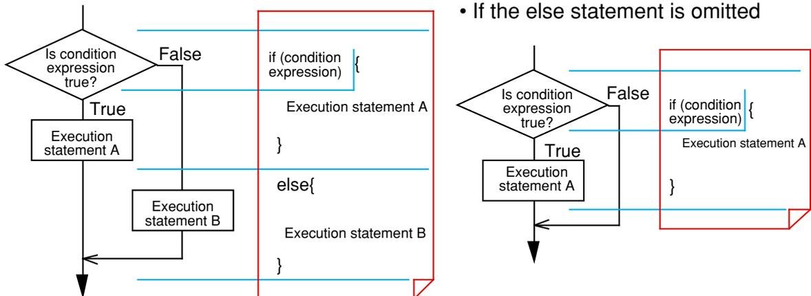
Figure 1.4.1 Example of "if-else" processing
