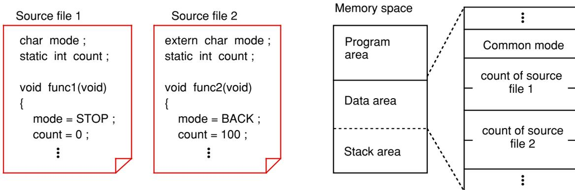
Figure 1.6.3 Storage classes of external variable
