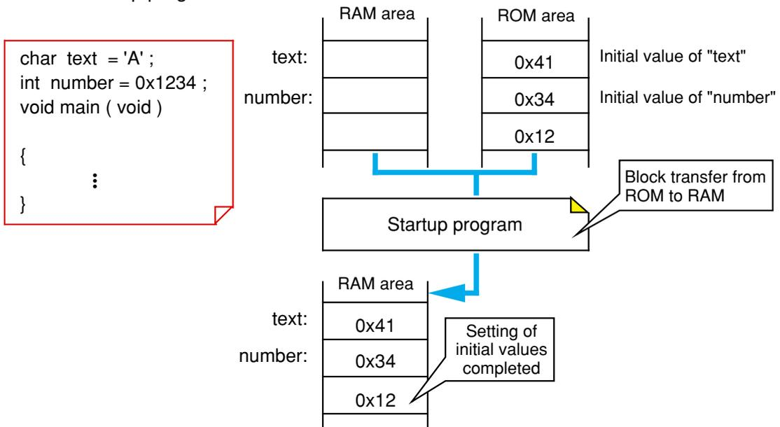
**Figure 2.1.2** Handling of static variables with initial values
