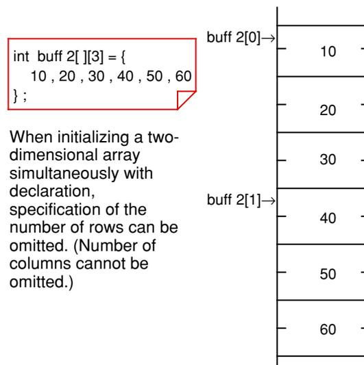
Figure 1.7.3 Declaration of two-dimensional array and memory mapping
