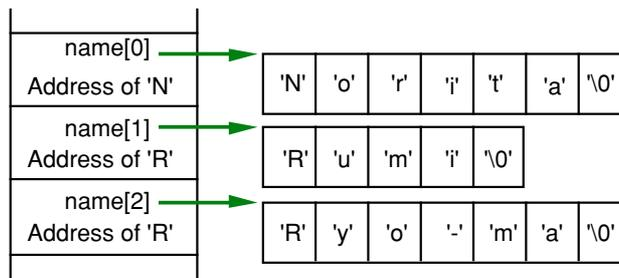
Figure 1.7.10 Difference between two-dimensional array and pointer array
