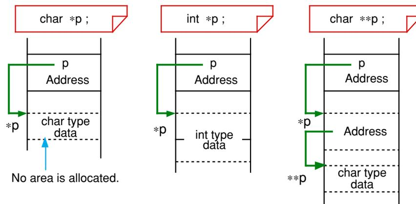
**Figure 1.7.4** Pointer variable declaration and memory mapping
