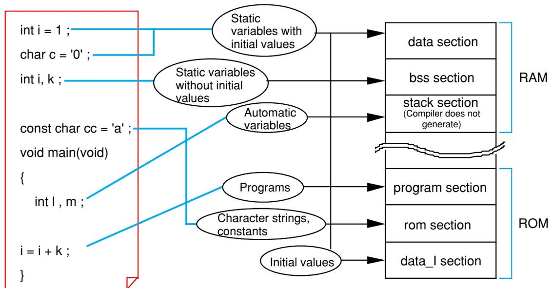
**Figure 2.1.3 Mapping data into sections by type**
