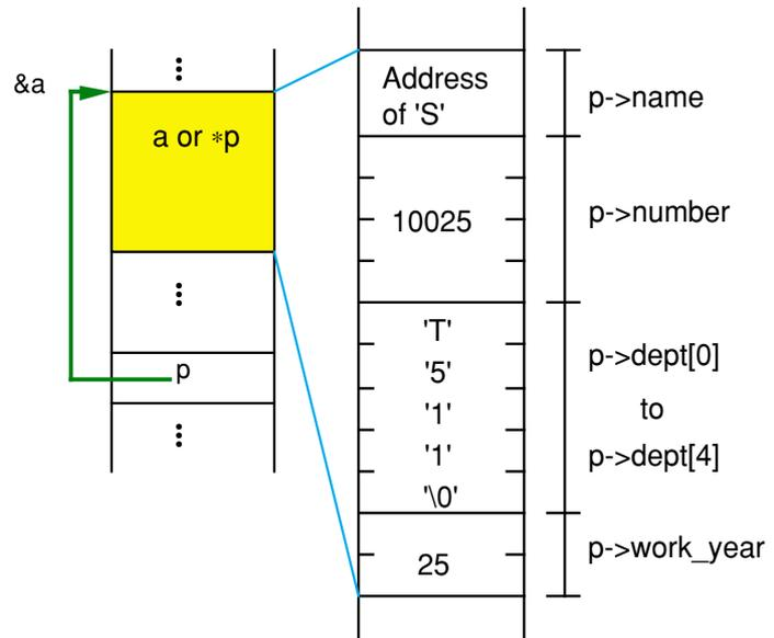
Figure 1.8.3 Example for referencing members using a pointer
