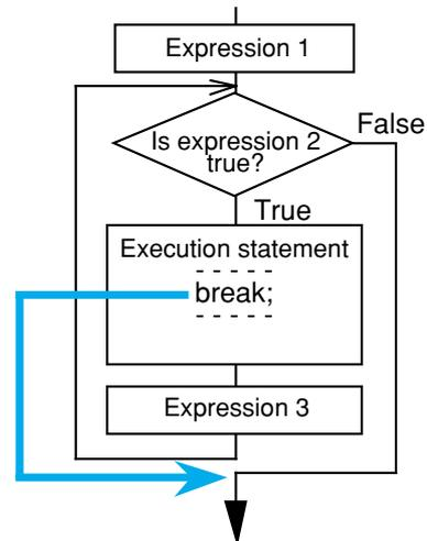
Figure 1.4.8 Example of "break" processing
