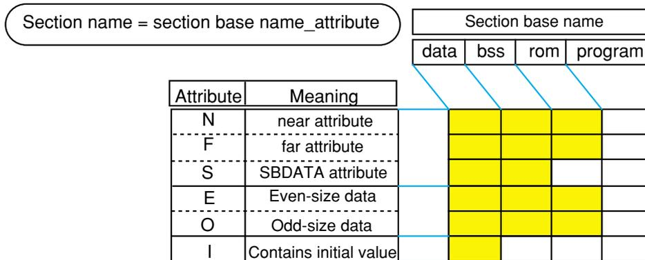
**Figure 2.1.4 Rule for assigning section names**
