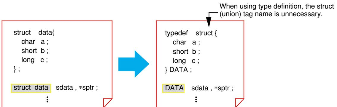
Figure 1.8.5 Example for using type definition "typedef"
