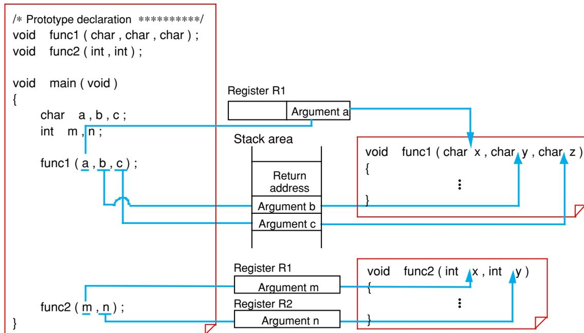
**Figure 2.4.4 Example for passing arguments to functions**
