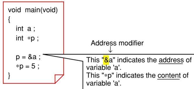
**Figure 1.7.5 Relationship between pointer variables and variables**
