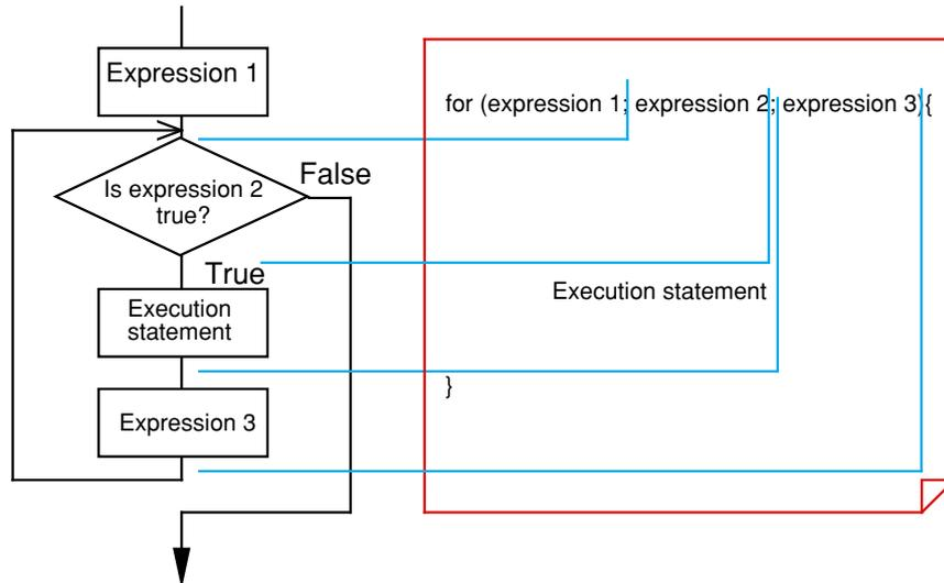
**Figure 1.4.6 Example of "for" processing**
