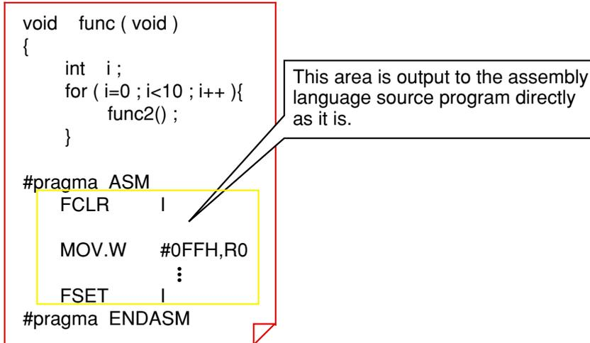
Figure 2.3.12 Example for using "#pragma ASM" function
