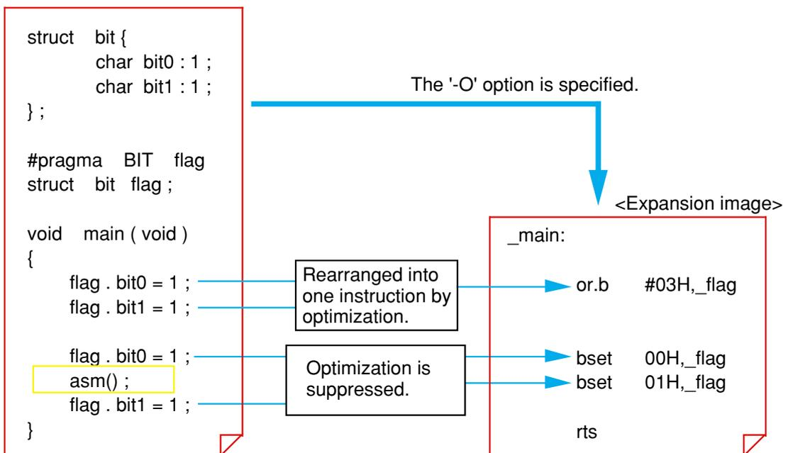
Figure 2.3.13 Suppressing optimization partially by using asm function
