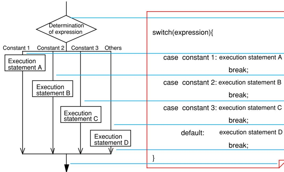
**Figure 1.4.3 Example of “switch-case” processing**
