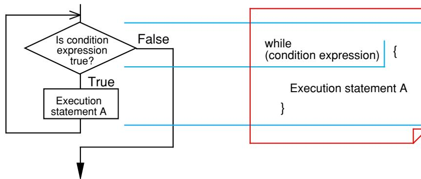
Figure 1.4.5 Example of "while" processing
