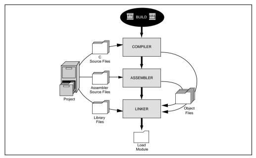
Figure 2.1: Typical Build Process
