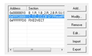
**Step 20:** After the "Modify section" dialog appears highlight and remove the section text "C\_1,C\_2,C,C\$\*,D\*,PResetPRG,P,W\*"
