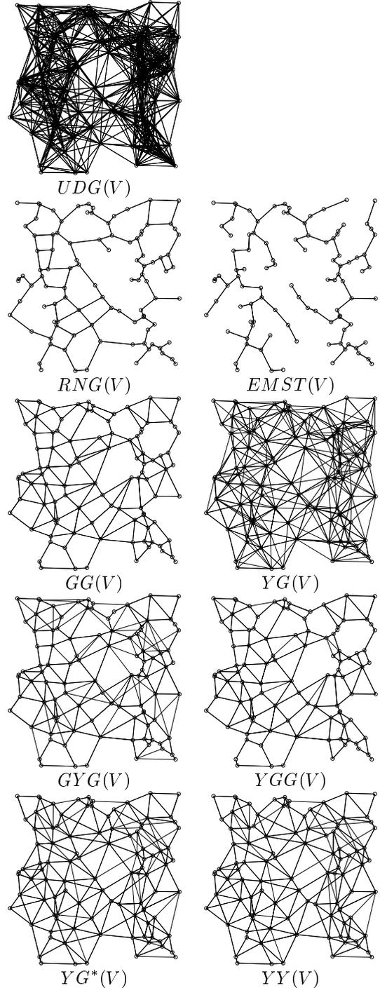
Figure 5: Different topologies generated from the same unit disk graph  $UDG(V)$ .
