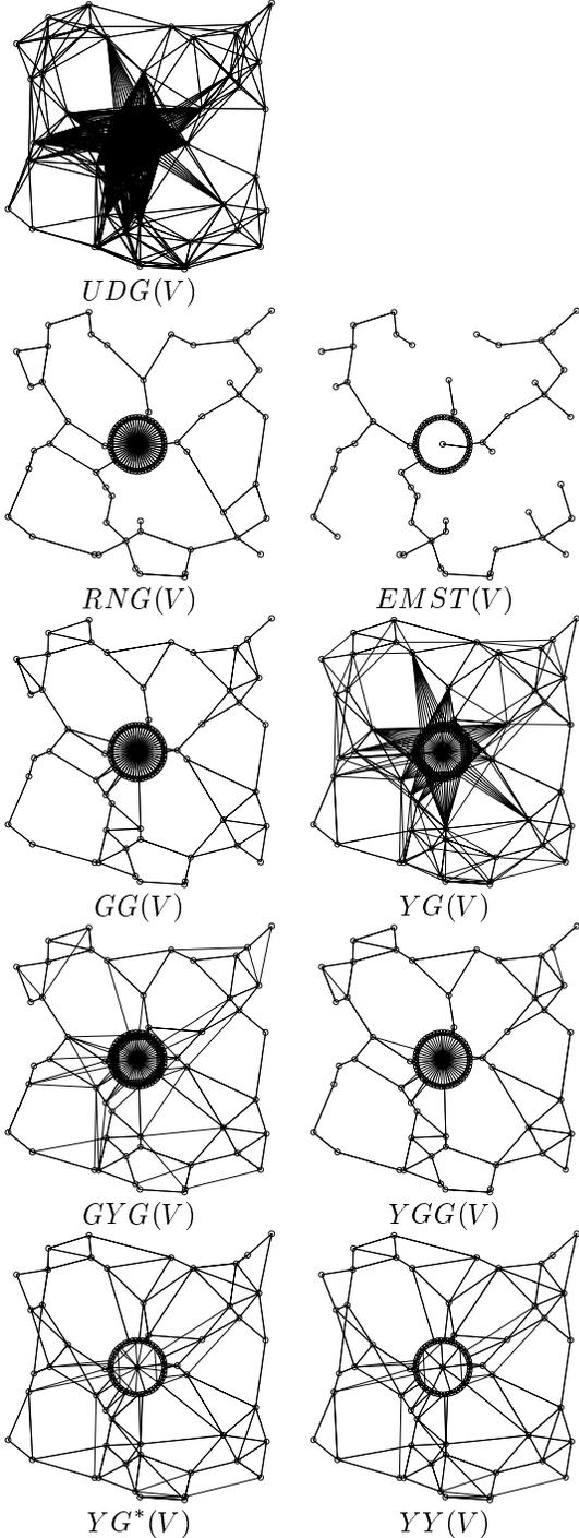
Figure 7: Different topologies generated from the same *unit disk graph*  $UDG(V)$ .
