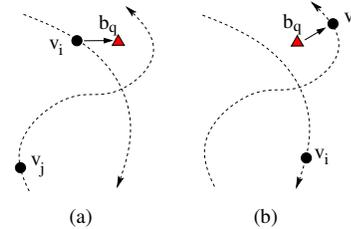
Fig. 1. Illustration of throwbox-assisted DTNs: (a) when a mobile node  $v_i$  passes by a throwbox  $b_q$ , it can left a copy of the message to  $b_q$ ; (b) later, throwbox  $b_q$  can then forward the message to another passing by node  $v_j$ .
