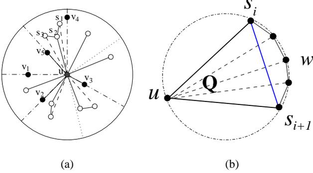
**Figure 1: (a) Constructing planar spanner with bounded degree for  $UDG(V)$ : process node  $u$ . (b) No new edges can be added by other nodes to intersect  $s_i s_{i+1}$ , where  $s_i s_{i+1}$  is added by  $u$  and not in  $UDel(V)$ .**
