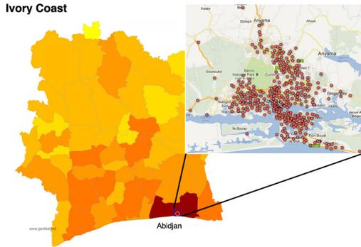
Fig. 1. **Visualization of D4D dataset:** the traffic distribution among all regions are shown in color where darker color indicates heavier traffic loads; the small blue rectangle around Abidjan shows the limited region with high traffic that we select for our simulations; and a zoomed view of the detailed tower distribution within the selected region is also provided.
