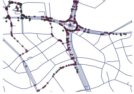
Fig. 4. The trajectories of one taxi with ID 18290 after interpolation within one hour. The green/pink points in the figure represent trajectory before/after interpolation.
