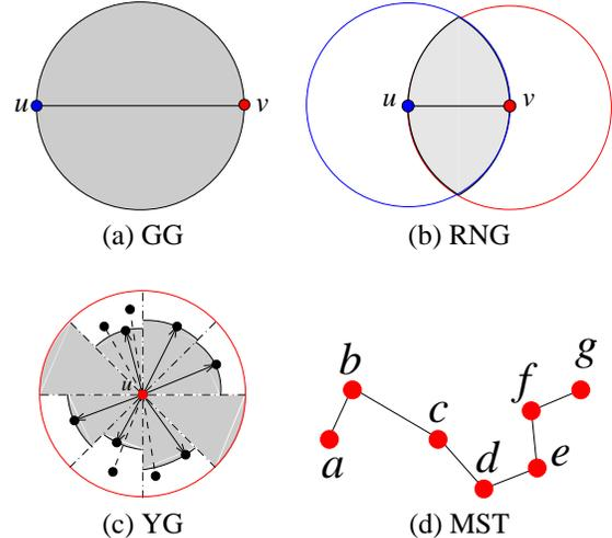
Fig. 1. The definitions of  $RNG$ ,  $GG$ ,  $YG$  and  $MST$ . The shaded area is empty of nodes inside.
