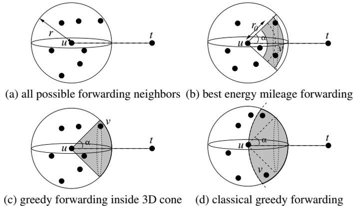
**Fig. 1.** Illustrations of our 3D routing: (a) energy-efficient forwarding in the restricted region, (b) greedy forwarding in the 3D cone, (c) greedy forwarding when the 3D cone is empty.
