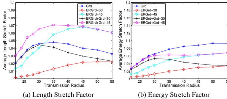
**Fig. 5.** Path efficiency (length stretch factor and energy stretch factor) of 3D ERGrd routing methods in random networks.
