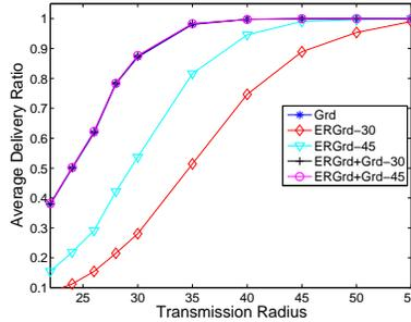
**Fig. 4.** Average delivery ratios of 3D ERGrd routing methods in random networks.
