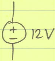
Independent Voltage Source (makes 12 volts)
