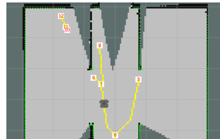
Fig. 5: Robot exploring the Straight Corridor Gazebo environment, moving along an edge of the skeleton graph. Skeleton graphs in Gazebo environments generate multiple vertices along the direction from the robot's current position to the exploration frontier. Here the vertices (7, 9, 8) are along the corridor. The skeleton graph shown here will be updated using the updated map after the robot reaches the target vertex. The frontier is the boundary between the light gray and dark gray regions of the map.
