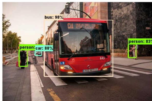
Figure 6. Example object detection results using MobileNet SSD.
