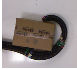
Fig. 1 A continuum manipulator wraps around a box.
