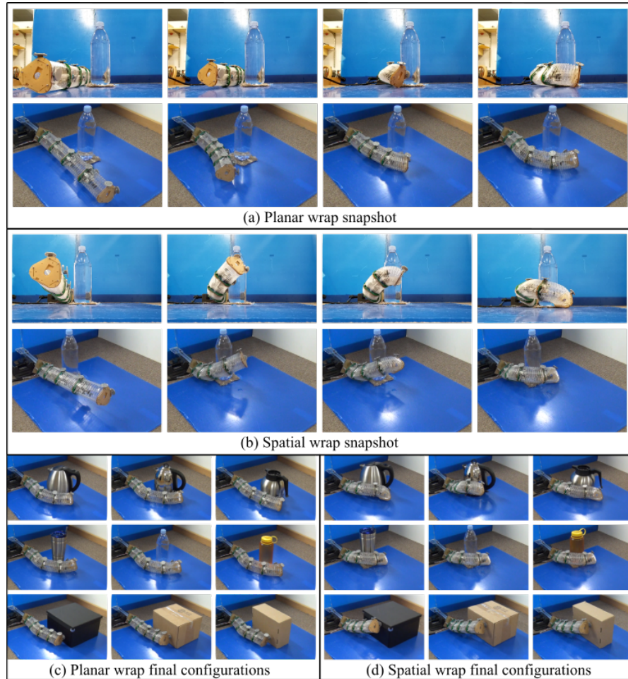
Fig. 5 The motion snapshots of (a) planar and (b) spatial continuum wraps around the bottle, where the top and bottom rows show the motion of the same wrap from two view angles respectively, (c) final configurations for the remaining objects with planar wraps, (d) spatial wrap final configurations.
