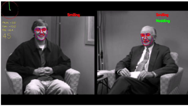
Fig. 1. Sample snapshots from tracked facial data showing a subject (left) and an interviewer (right). Red dots represent tracked facial landmarks (eyes, eyebrows, etc.), while ellipse in top left corner depicts the estimated 3-D head pose of the subject; top right corners show the detected expressions, and head gestures for subject and interviewer.
