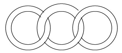
(B) Look at the diagram, and note the length of a chain with n links is 2R + 2(n-1)r where R is the outer radius and r is the inner radius. Thus, 2R + 2r = 13 and 2R + 4r = 18, which yields 2r = 5/2 and 2R = 8. Thus the length of a 25 link chain is 2R + 24r = 8 + 120 = 128. Alternatively, note that each link adds 5 cm. to the length of the chain, for a total of  $8 + 5 \cdot 24 = 128$ .
